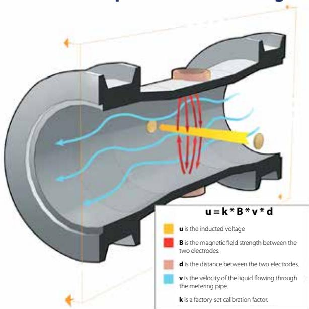
The principle of operation is based on Faraday's law of electromagnetic Induction. A highly accurate, bipolar pulse circuitry energizes two coils - creating a magnetic field perpendicular to the direction of the flow.
